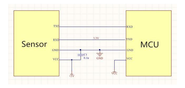
Picture 1: UART Communication Connecting Circuit
