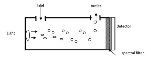
Basic mathematical model: A majority of both organic and inorganic polyatomic gas have specific absorptive wavelength in infrared region. When infrared light passed by, the light transmissivity of this gas molecule to certain wavelength can be expressed by Lambert-Beer Law:
