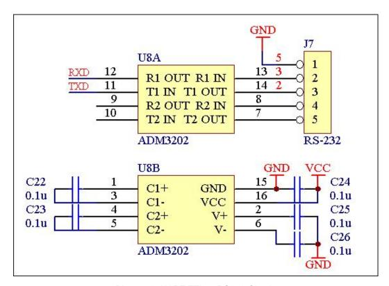
Picture 2: UART-TTL to RS232 Circuit
