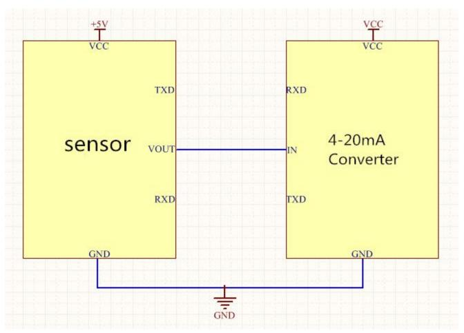
Picture 4: Analogue signal output circuit
