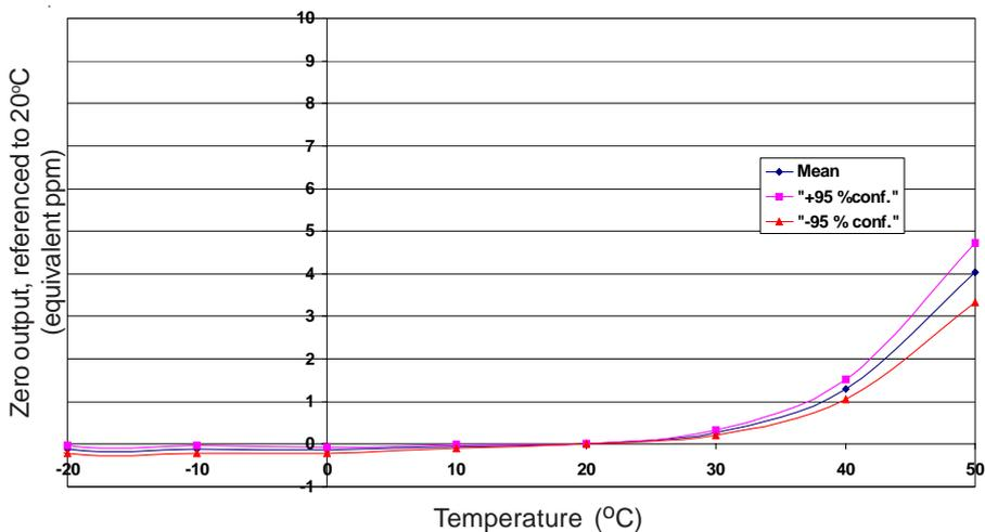
Figure 3 shows the variation in zero output caused by changes in temperature expressed at ppm gas equivalent.
