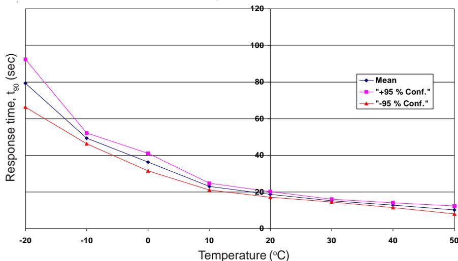
Sensor response time increases as temperature decreases. Alphasense response time ( $t_{90}$ ) is quoted at 20°C.
