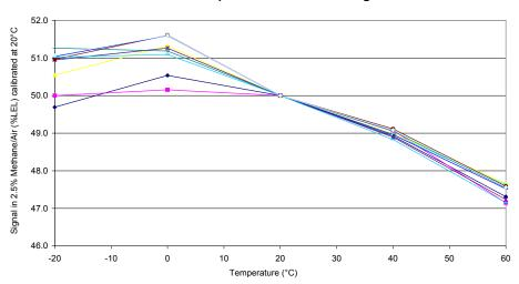
Effect of Temperature on Zero Signal
