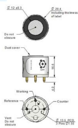
All tolerances ±0.15 mm unless otherwise stated. DO NOT solder to pins.
