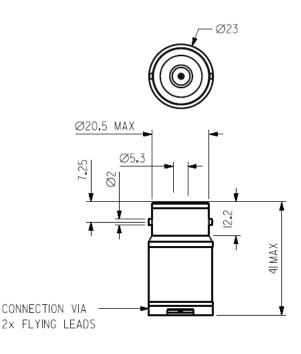
$\label{eq:all dimensions in mm.} All \mbox{ dimensions in mm.} \\ All \mbox{ tolerances } \pm 0.15 \mbox{ mm unless otherwise stated} \\$
