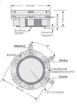
All dimensions in mm All tolerances ±0.15 mm unless otherwise stated 3NFF shown with side tags and tin pins
