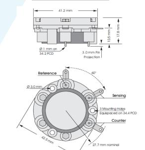
All dimensions in mm All tolerances ±0.15 mm unless otherwise stated 3FF shown with side tags and tin pins
