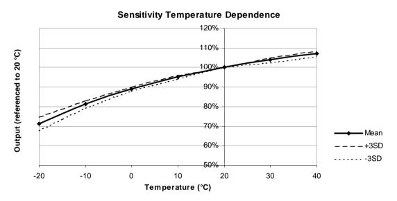
Figure 1: Sensitivity dependence expressed as a percentage of the signal at 20 °C. The result is shown along with confidence intervals corresponding to ±3 times the standard deviation.
