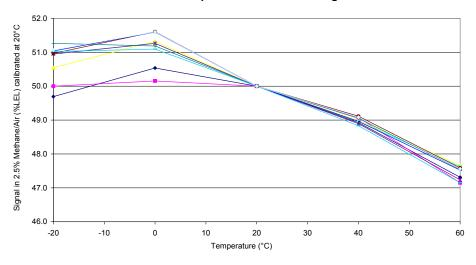
Effect of Temperature on Zero Signal
