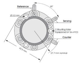
All dimensions in mm All tolerances ±0.15 mm unless otherwise stated 3FD shown with side tags and tin pins
