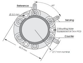
All dimensions in mm All tolerances ±0.15 mm unless otherwise stated 3MF shown with side tags and gold pins
