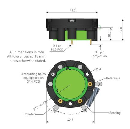
$\label{lem:lem:portant note:} \textbf{IMPORTANT NOTE:} \ \textbf{Connection should be made via PCB sockets only.} \ \textbf{Soldering to the pins will seriously damage your sensor}$
