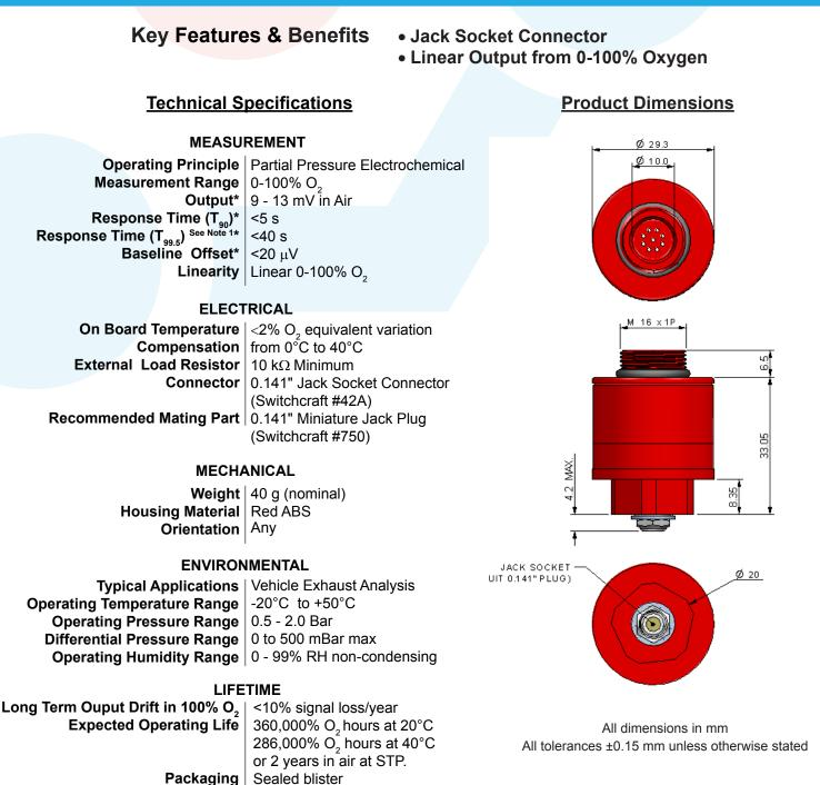
**Note 1:**  $T_{99.5}$  Response is equivalent to a change in concentration fom 20.9% O<sub>2</sub> to 0.1% O<sub>2</sub>
