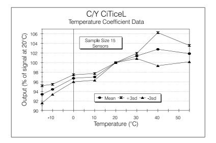
Performance characteristics on this data sheet outline the performance of newly supplied sensors. Output signal can drift below the lower limit over time.
