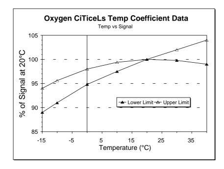
Performance characteristics on this data sheet outline the performance of newly supplied sensors. Output signal can drift below the lower limit over time.
