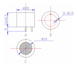
A-Left view B-upward view C-vertical view W electrode — working electrode for oxidation reaction C electrode —counter electrode for deoxidization reaction
