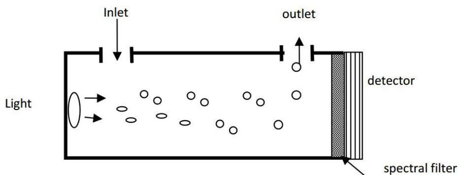
Basic mathematical model: A majority of both organic and inorganic polyatomic gases have specific absorptive wavelengths in the infrared region. When infrared light passes through, the light transmissivity of this gas molecule to a certain wavelength can be expressed by Lambert-Beer's Law:
