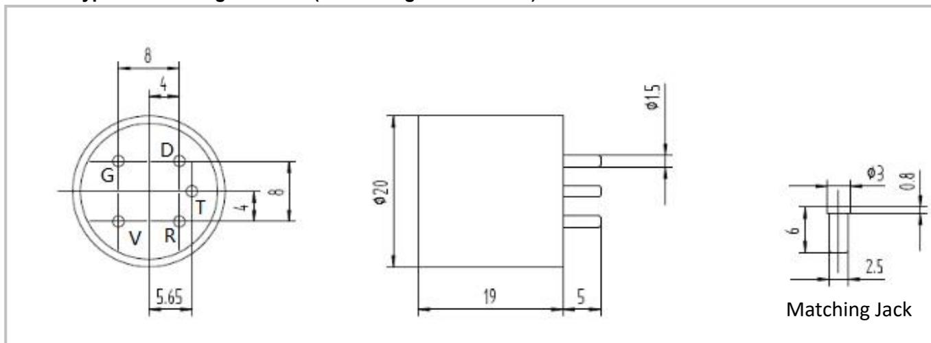
SXH-XB Type Sensor Height 16.6mm (See Configuration Table)
