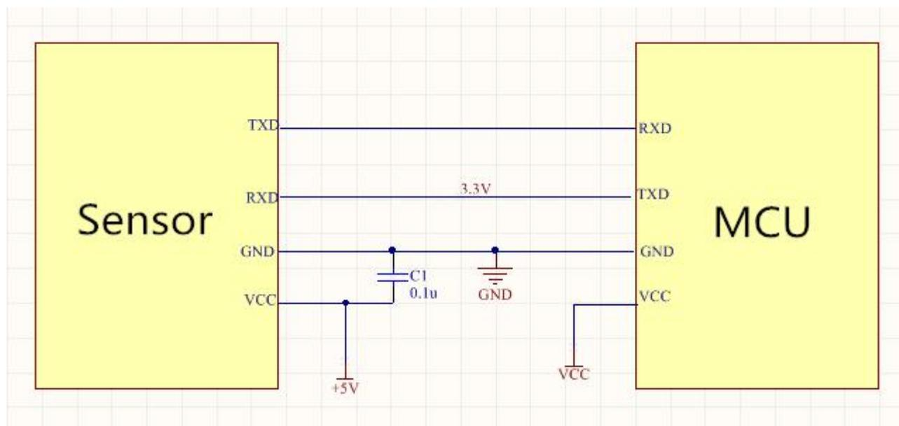
**Picture 1:** UART Communication Connecting Circuit
